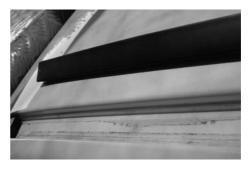
Place the Track over the exposed gutter 65mm from the front windscreen. There is a left and a right track. The bend in the Track should be to the front and facing the outside of the vehicle.
