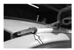
( **F** ) Mark position of the holes in the Track onto the vehicles roof with a marking pen. There will be four holes per track.
