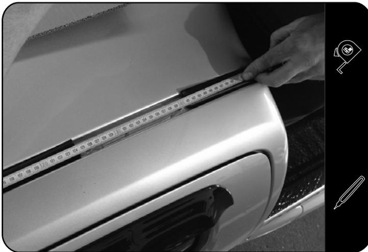
Still measuring from the front windscreen mark the Ditch Moulding at the following distances 1245 mm and 1410 mm.
