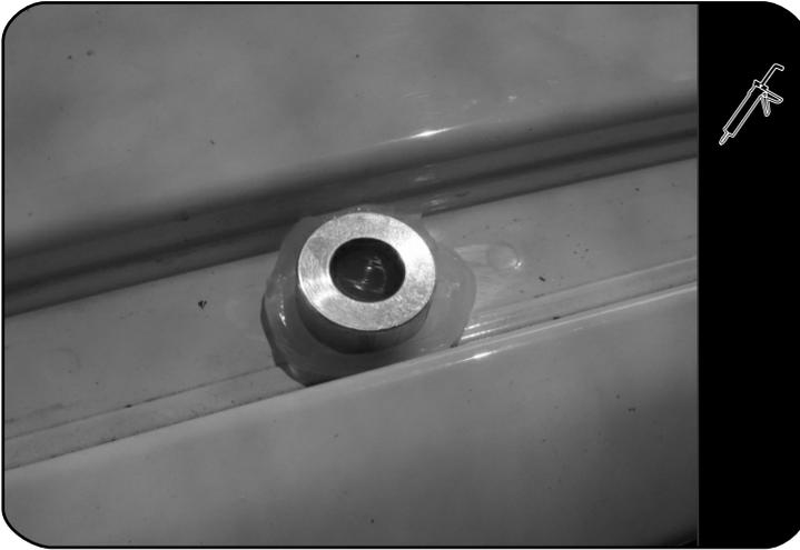
Put a small amount of silicone over each Mounting Point and place a Spacer (Item 9) on top of the Silicone, lining up the hole in the Spacer with the mounting point.
