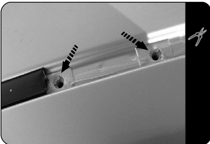
Using a pair of tin snips, cut the Ditch Moulding on each of your marks and remove the small strips of Ditch Moulding between markings 1-2 and 3-4.
