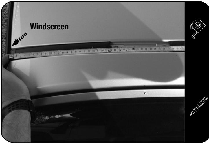
Starting at the front windscreen as shown, measure along the Ditch Moulding towards the rear of the vehicle. Mark the Ditch Moulding at the following distances 240mm and 375mm.
