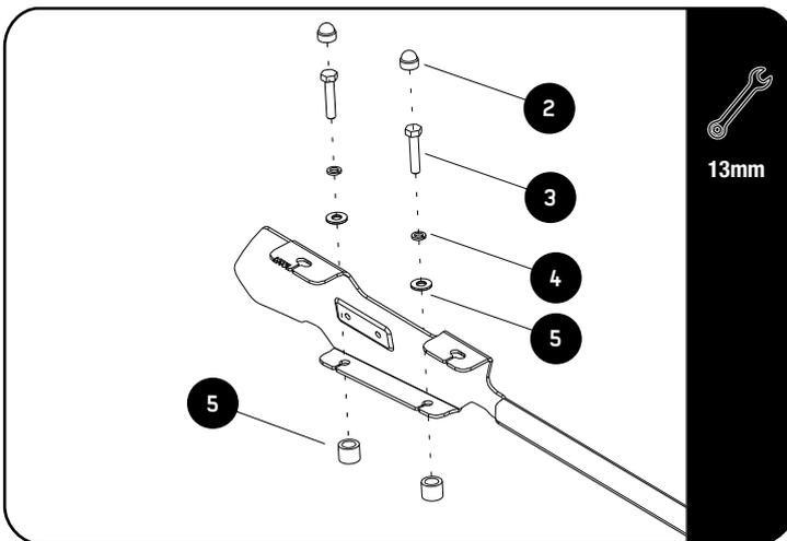
Place the Foot Rail (Item 1) onto the Spacers, aligning the holes in the base of the Foot Rail with the center of the Spacers. The product sticker goes to the front of the vehicle and must face outwards.
