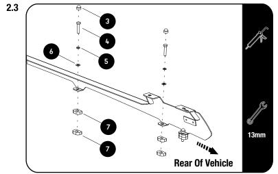
Place a bead of silicone around each of the M8 x 40 Hex Bolt threads.
