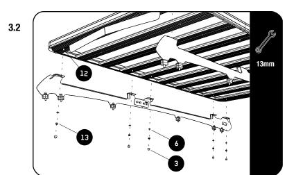
Fit your Roof Rack to the Foot Rails using M8 x 20 Hex Bolts, M8 x 16 x 1.6SS Flat Washers and M8 Nyloc Nuts (Items 6, 12 & 13).
