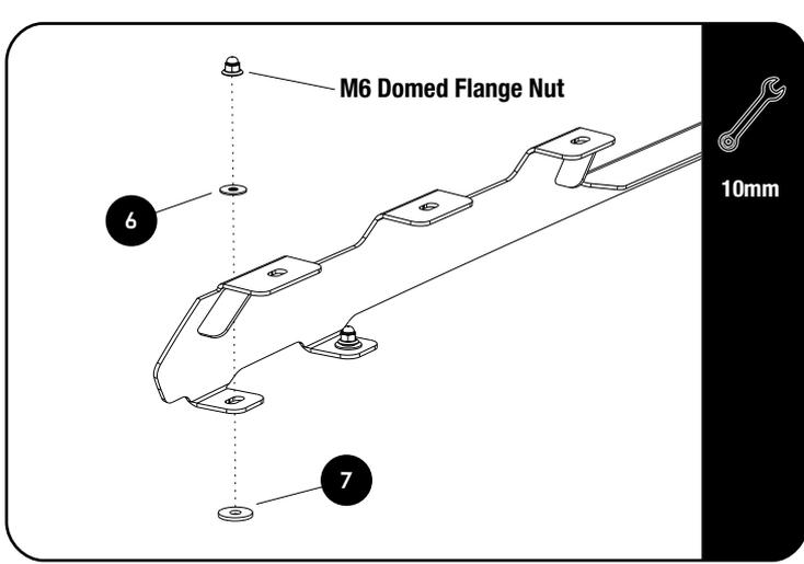
Place a PVC Washer (Item 7) over each of the studs in the vehicle's roof followed by the Foot Rail.
