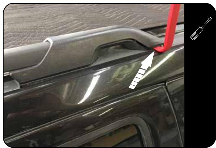
Before starting the fitment you need to remove the factory rails. Start by removing the front and rear rail covers using a panel tool or similar.
