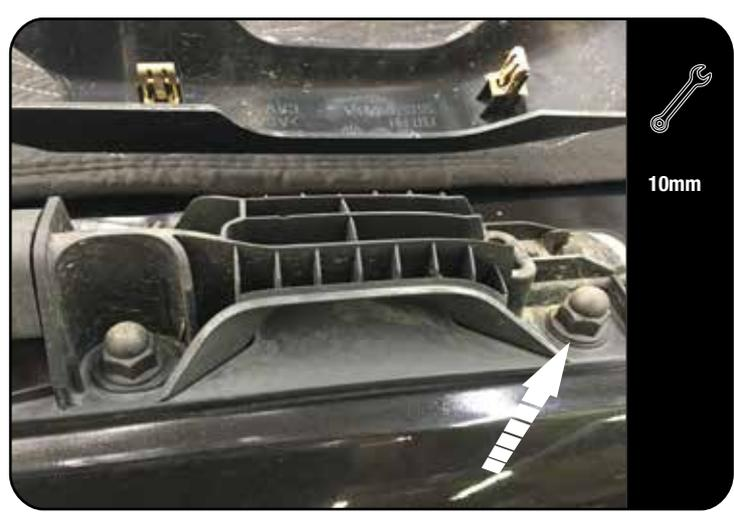
Loosen and remove the M6 Domed Flange Nuts. Keep them in a safe place as you will reuse them to fit the Front Runner Foot Rails.
