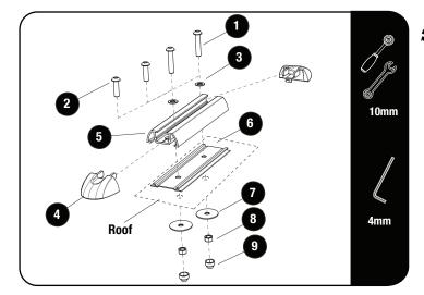
Fit and secure the tracks with a combination of items 1/2, 6, 7, 8.
